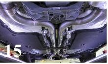
WARNING: Use extreme caution during installation. Torque all fasteners according to manufacturer's torque values and tightening sequence. <u>DO NOT</u> use air impact tools to tighten fasteners on Borla Performance Exhaust Systems. Use of such tools may result in bent flanges or gasket contact areas leading to exhaust leaks.
