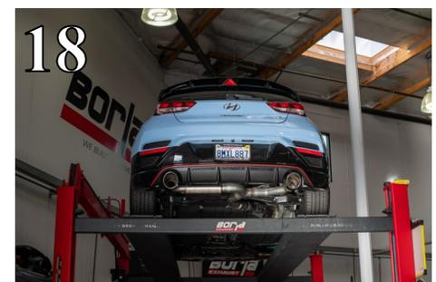
**WARNING:** Use extreme caution during installation. Torque all fasteners according to manufacturer's torque values and tightening sequence. **DO NOT** use air impact tools to tighten fasteners on Borla Performance Exhaust Systems. Use of such tools may result in bent flanges or gasket contact areas leading to exhaust leaks.
