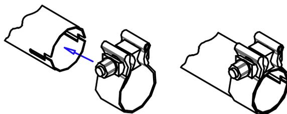
**WARNING:** Use extreme caution during installation. Torque all fasteners according to manufacturer's torque values and tightening sequence. **DO NOT** use air impact tools to tighten fasteners on Borla Performance Exhaust Systems. Use of such tools may result in bent flanges or gasket contact areas leading to exhaust leaks.
