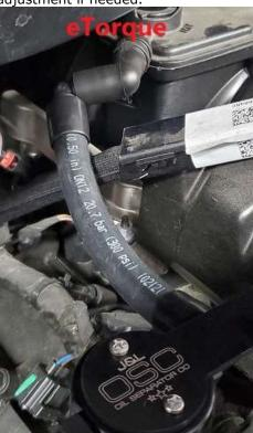
The J&L bracket is going to sandwich between the engine cover and engine cover mounting stud. Reinstall engine cover into rear grommets. Feed bolt into engine cover and J&L Mounting bracket, if you look from the front of the engine, you will be able to see the bolt location to help align it back into the mounting hole. Start bolt by hand and tighten with ratchet.
