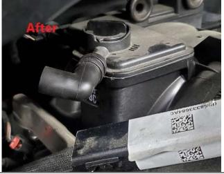
Install J&L Oil separator onto J&L mounting bracket with supplied screws. Logos on bracket and can should line up.
