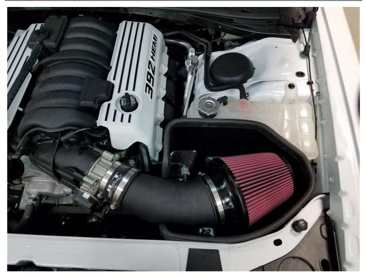
Oil Filter: The frequency you should clean your filter will depend on your driving conditions. It is recommended to check your filter at every oil change or 3,000 miles. If there is a buildup of dirt as thick as the wire mesh, then it's time to clean your filter. To properly clean your oil filter, we recommend the S&B Precision Cleaning & Oiling Kit (located in the Parts Sold Separately Section of our website, www.JLTtruecoldair.com).
