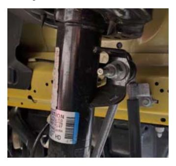
5. Using a 15mm socket remove the two caliper to spindle bolts holding on the caliper. Do not let the caliper drop or hang from the brake hose. We recommend securing it the brake hose to chassis bracket like shown in the photo.
