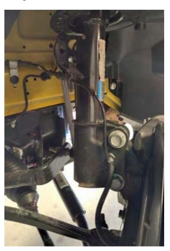
4. Remove the front anti-sway bar link from the strut housing. DO NOT USE AN IMPACT GUN. Do this by using a 17mm wrench on the flats of the stud and using a 18mm socket to remove the nut.
