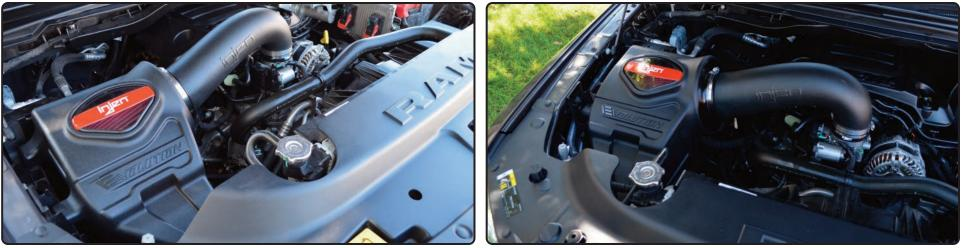
Congratulations! You have just completed the installation of this intake system. Periodically, check the alignment of the intake, normal wear and tear can cause nuts and bolts to come loose. <u>Note: Check clearance and adjust if needed! Failure to check</u> the alignment and adjust the intake can cause damage that will void the warranty. Injen Technology is not responsible for any damages caused by/from improper installation.
