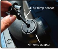
**14.** Install the temperature sensor into the adaptor. twist and lock into place.
