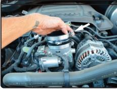
**10.** Install the provided 3.5" hump hose with clamps to the throttle body. Secure and tighten on the throttle body only.
