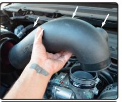
**15.** Install the intake tube and position the intake tube to the filter and the tube to the throttle body.
