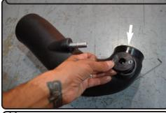
**11.** Install the temp sensor adaptor to the tube and secure using provided M4 button head screws.
