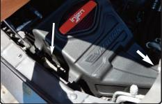
8. Install the air box assembly into the truck and position the air box to the studs from the OEM air box. Make sure the front of air box is seated properly. Page 3 EVO8101
