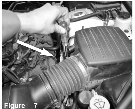
Figure 7 Loosen the clamp on the air box.
